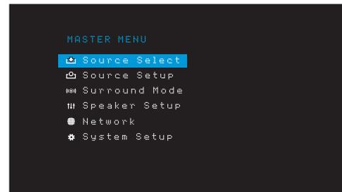
4. Use the remote's arrow and OK buttons to select "Source Setup," and use the left/right arrow buttons to select a source button with connectors that you want to re-assign.
