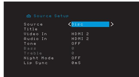
5. Select "Video In" and select the video input connector you want to assign to the source button. Press the OK button. **NOTE:** If you select an HDMI connector as the video input connector, the audio input connector will automatically change to the same HDMI connector. You cannot use a different audio input connector with an HDMI video input connector.
