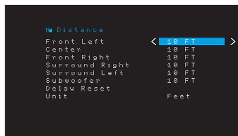
Enter the distance from each speaker to the listening position that you measured in Step Two and recorded in Table A3 in the Appendix (see page 33). Select a speaker, then use the Left/Right buttons to change the measurement. You can enter distances between 0 and 30 feet (9.1m). The default distance for all speakers is 10 feet (3m).
