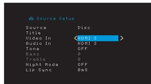
6. If you have not selected an HDMI connector for Video In, select “Audio In” and select the audio input connector you want to assign to the source button. Press the OK button.
