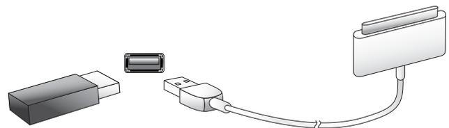
**IMPORTANT: Do not connect a PC or other USB host/controller to the AVR's USB port, or you may damage both the AVR and the other device.**
