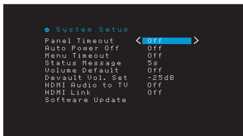
**Panel Timeout:** This setting allows you to set the AVR's front-panel display to automatically turn off after remaining on for a predetermined time (3 – 10 seconds) each time you use a control. Set this to "Off" to have the display remain on continually.
