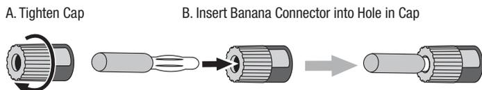
Always connect the colored (+) terminal on the AVR to the (+) terminal on the speaker (usually red), and the black (-) terminal on the AVR to the (-) terminal on the speaker (usually black).
