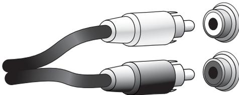
For source devices that have both digital and analog audio outputs, you may make both connections.
