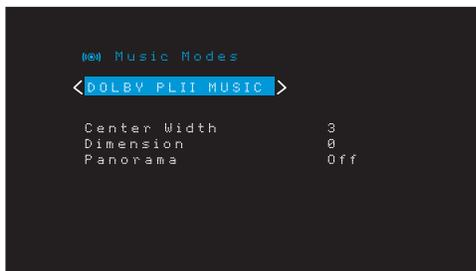
**Center Width:** This setting affects how vocals sound through the three front speakers. A lower number focuses the vocal information tightly on the center channel. Higher numbers (up to 7) broaden the vocal soundstage. Use the Left/Right buttons to adjust.
