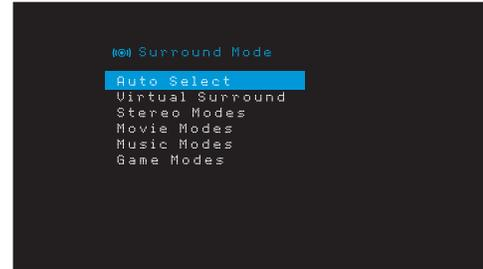
**Auto Select:** For digital programs, such as a movie recorded with a Dolby Digital or DTS soundtrack, the AVR will automatically use the soundtrack's native surround format. For two-channel analog and PCM programs, the AVR uses the Logic 7 Movie or 2CH Stereo mode, depending on the source.
