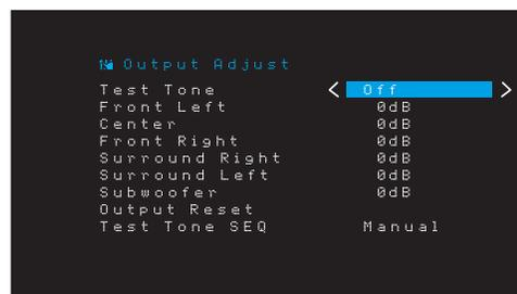
All of the system's speakers will appear with their current level settings. You can adjust each speaker's level between -10dB and +10dB in 1dB increments.
