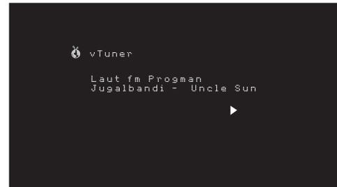
With the vTuner screen (above) displayed, the AVR will automatically connect to the Internet via the [www.radioharmanardon.com](http://www.radioharmanardon.com) portal. To select a stream use the Up/Down buttons to search by category. **NOTE:** The categories displayed vary by region.
