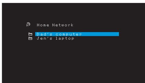
The screen will list by name all devices on the network that allow sharing. Use the Up/Down and OK buttons to browse the content stored in the device’s media player library. Scroll to the desired item and press the OK button to select it. To return to the previous menu level (or to clear the menu from view from the top level), press the Back/Exit button.
