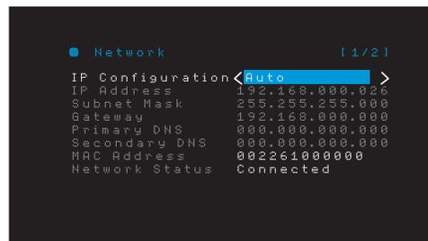
3. Select IP Configuration, then press the Right button twice to cycle the setting from “Auto” to “Manual” and back to “Auto.”
