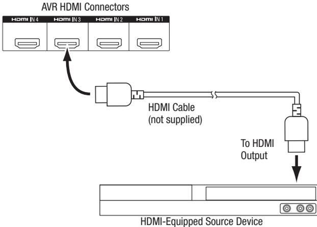
**NOTE:** If you have HDMI devices already connected directly to your TV, you can feed their sound to the AVR via the HDMI Out connector's Audio Return Channel, and they will not require additional connections to the AVR.
